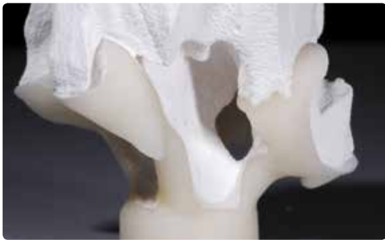
Fine divestment is carried out with polishing beads at 2 bar (29 psi) pressure.
