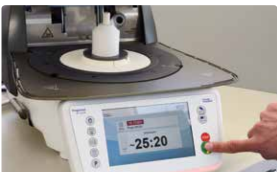
Place the loaded hot investment ring in the centre of the preheated press furnace using the investment ring tongs. Press START to start the IPS e.max Press Multi program.
