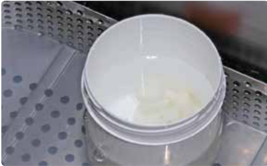
Remove the reaction layer formed on the pressed objects using the Invex Liquid in an ultrasonic bath.
