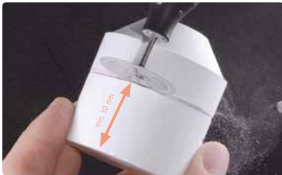
Separate the investment ring at a distance of at least 30 mm from the bottom surface using a separating disc...
