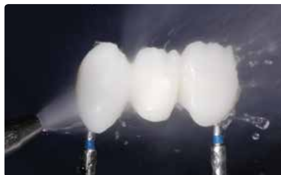
Blast the restoration with Al 2 O 3 (type 100) at 1 bar (15 psi) pressure. Thoroughly clean the surface with a steam jet prior to the Wash firing and subsequently dry.
