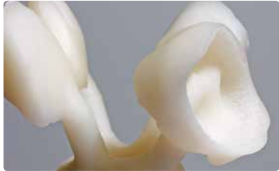
Remove the reaction layer formed on the pressed objects using the Invex Liquid in an ultrasonic bath.
